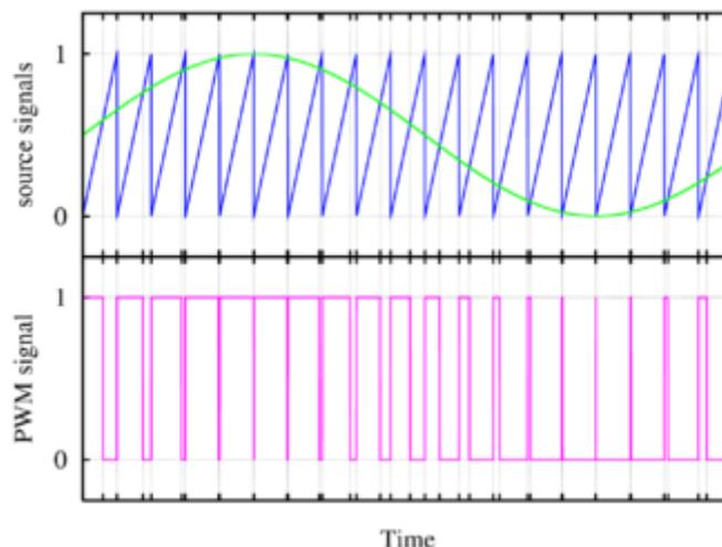
**Fig. 4 Pulse Width Modulation Signal Graph**
