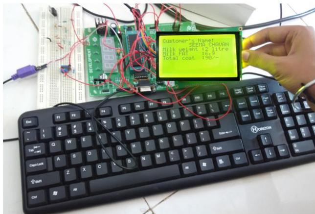
**Fig. 4 Interfacing keyboard and GLCD with pic**
