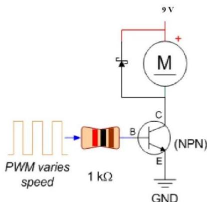
**Fig 3. Driver circuit**
