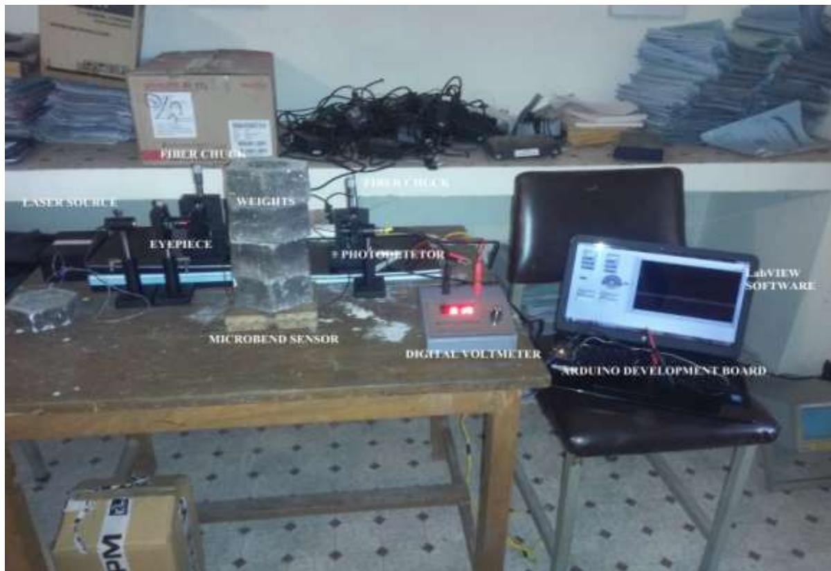
Figure 9: Picture of the experimental set-up
