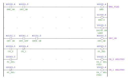
Figure 3: Introductory Ladder programming
