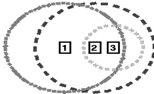
**Fig 3 Ad hoc network with a one-way link**
