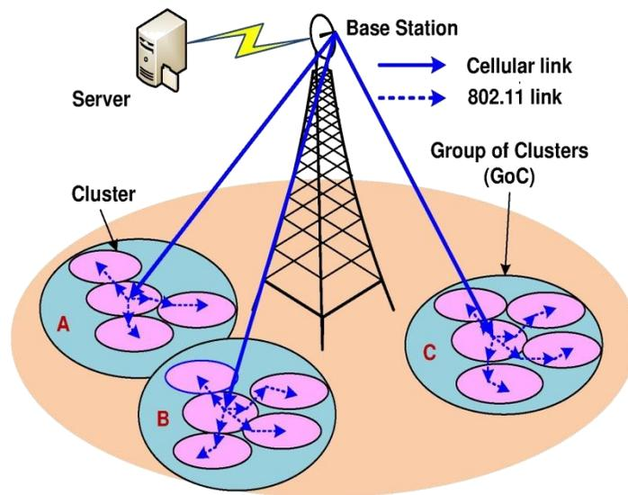
**Fig1: Shows That the Block Diagram of a Hybrid Cellular and Network Links**
