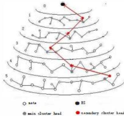
**Fig. 3: Double cluster head selection method [4]**
