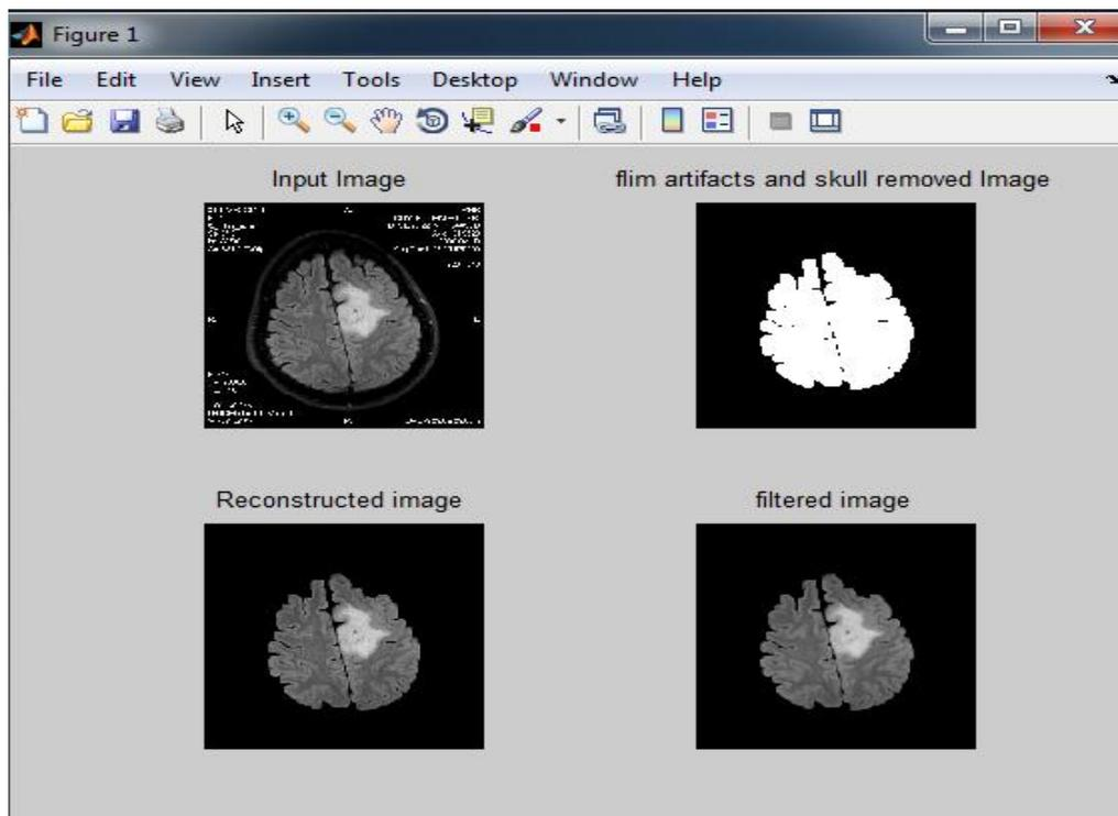
**Fig.2 Screenshot for Output of pre-processing stage**
