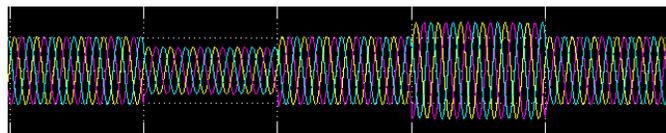
**Fig.7 Supply Voltage Having Voltage Sag & Swell**
