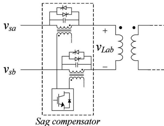
**Fig.2 Connection diagram of the proposed system with delta/bye load transformer.**
