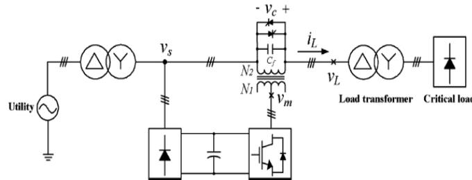
**Fig.1 single-line drawing of the offline series voltage sag compensator.**
