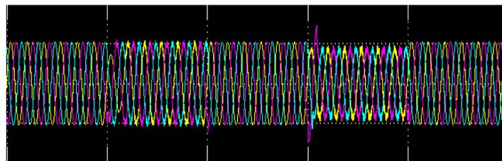
**Fig.8 voltage across sensitive load after voltage injection**
