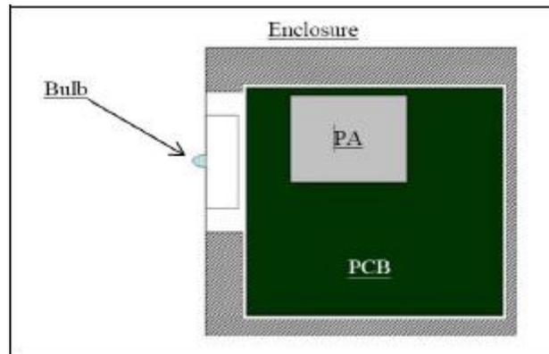
The PCB controls the electrical inputs and outputs of the lamp and houses the microcontroller used to manage different lamp functions. A RF (radio-frequency) signal is generated by the solid-state Power Amplifier and is guided into an electric field about the bulb. The high concentration of energy in the electric field vaporizes the contents of the bulb to a plasma state at the bulb's centre; this controlled plasma generates an intense source of light.
