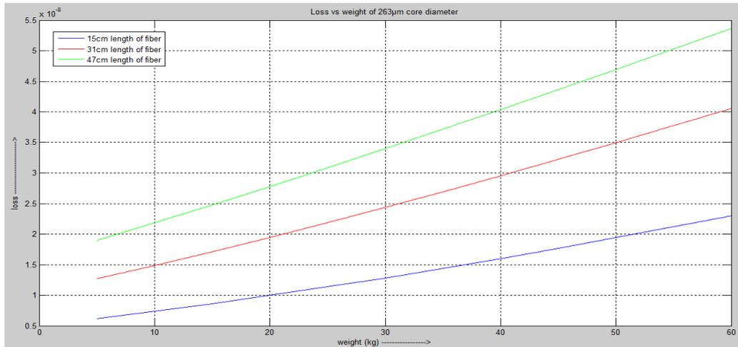
**Figure 6: Loss Vs Weight Comparison Curve of Different Lengths of Optical Fibers of 263µm Core Diameter Optical Fiber**
