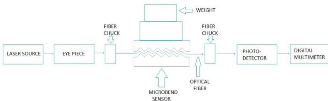
Figure 3: Schematic diagram of weight measurement
