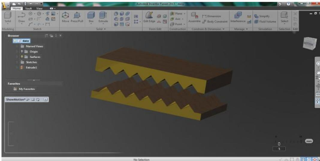
Figure 1: Microbend sensor design in AutoCAD
