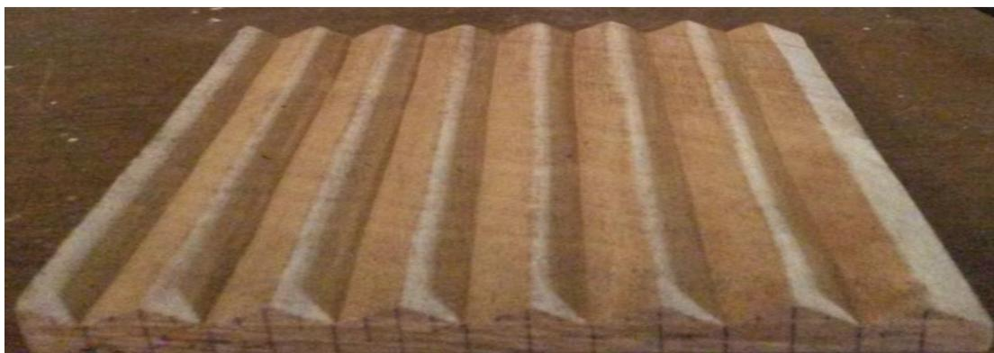
Figure 2: Picture of one plates of the designed microbend sensor
