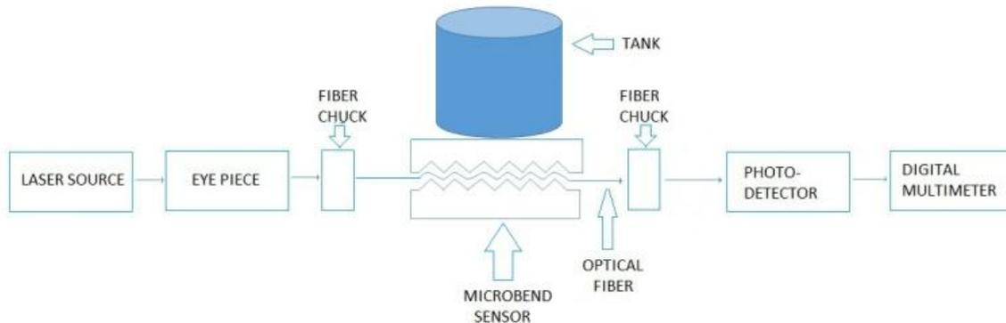
**Figure 4: Schematic diagram of liquid volume and level measurement**
