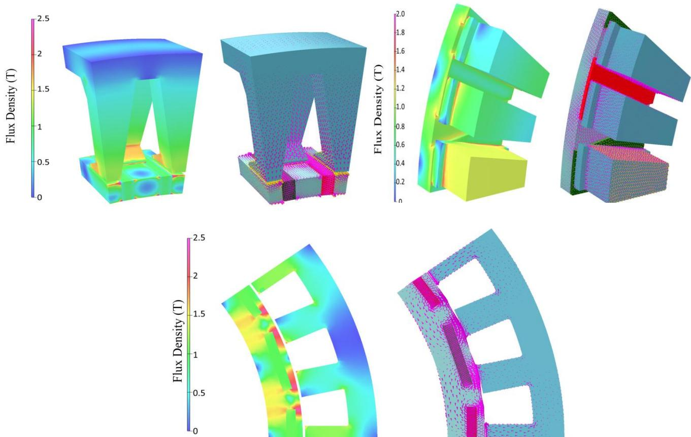
**Fig. 6. Field distribution and flux density vectors of CPTFM (upper), SAT (middle) and RFPM (lower) with no-load**
