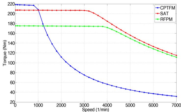
Fig. 9. Speed-Torque-Curve of CPTFM, SAT and RFPM with constant J
