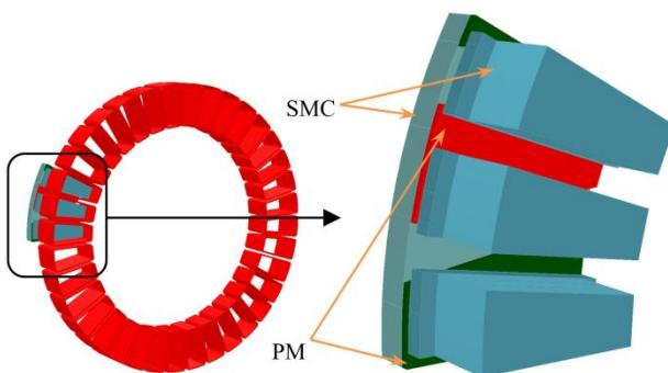
Fig. 3. Model of AFPM in FEM
