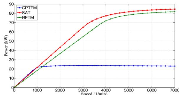
Fig. 10. Speed-Power-Curve of CPTFM, SAT and RFPM with constant J
