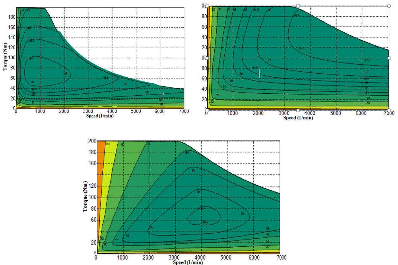
**Fig. 12. Efficiency Maps of CPTFM (upper), SAT (middle) and RFPM (lower)**
