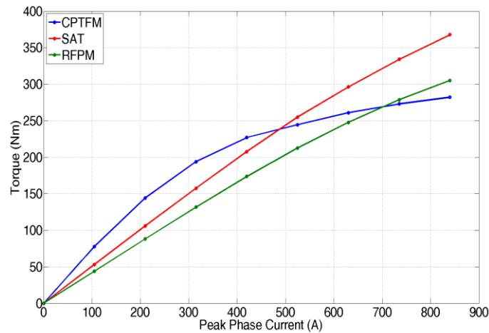
Fig. 8. Average Torque of CPTFM, SAT and RFPM
