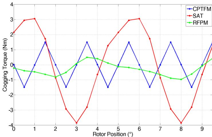
**Fig. 7. Cogging Torque of CPTFM, SAT and RFPM**
