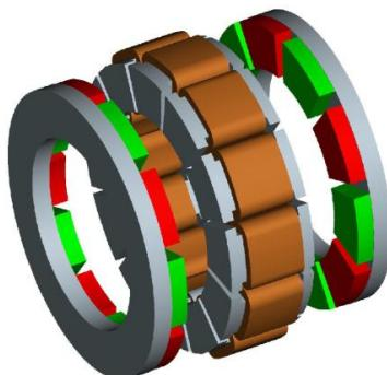
Fig. 2. Model of segmented armature torus machine
