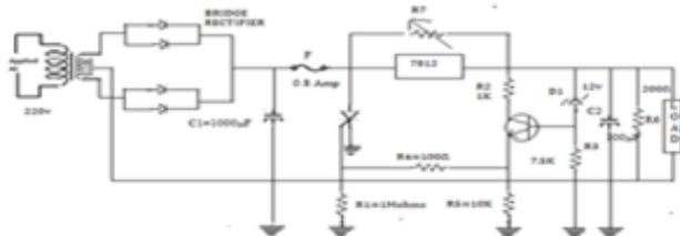
**Fig. 1 Over voltage protection using SCR as a crowbar Device**
