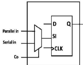
**Fig. 4. Dual muxed scan flop**
