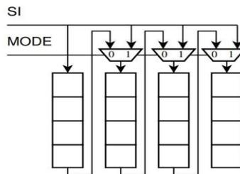
**Fig. 1. Illinois scan architecture**
