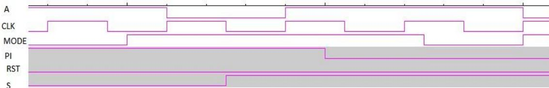
**Fig. 10. Muxed scan flop output**
