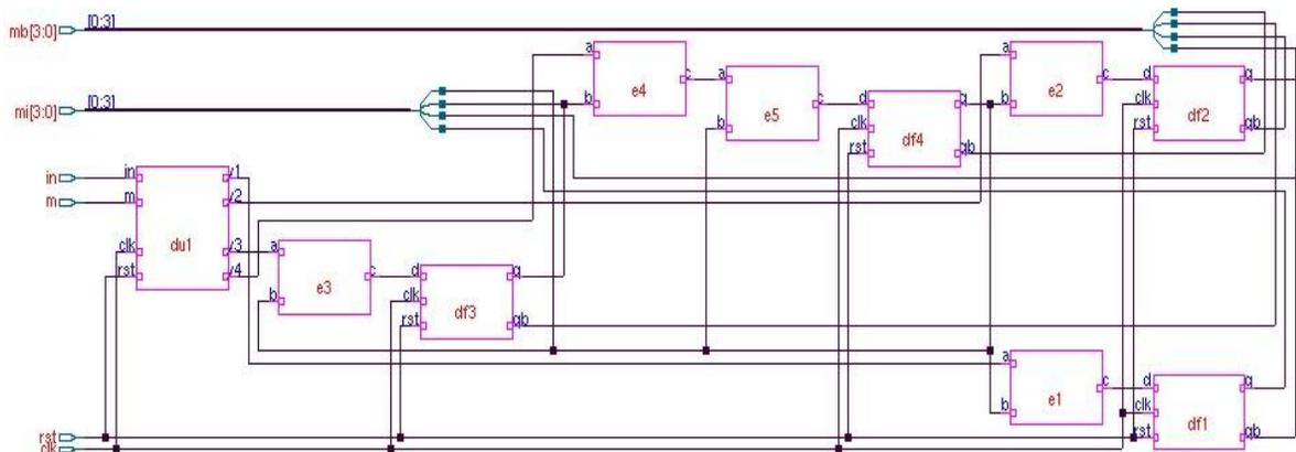
**Fig. 11. Illinois Scan Chain RTL**
