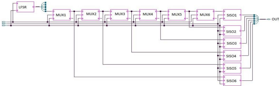
**Fig. 13. Broadcast Architecture RTL**
