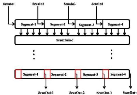
**Fig. 3. Segmented Broadcast architecture**
