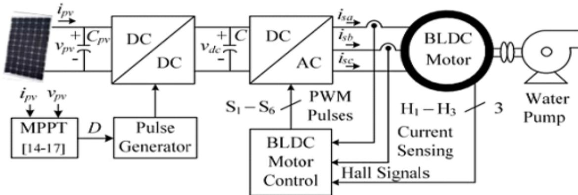
**Fig. 1 Conventional SPV fed BLDC motor driven water pumping system.**
