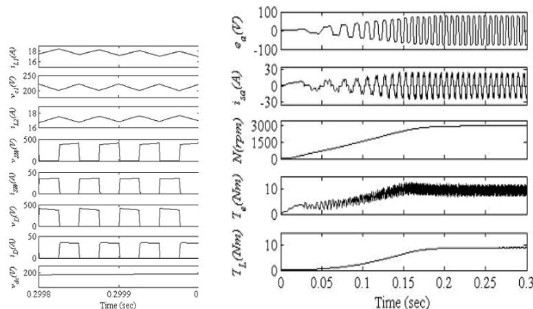
**Fig.4 Starting and steady state performances of the proposed SPV array based Zeta converter fed BLDC motor drive for water pump (a) SPV array variables, (b) Zeta converter variables, and (c) BLDC motor-pump variables.**
