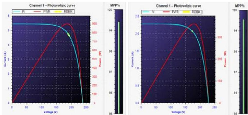
Fig. 6 (a) (b) MPPT performance at (a) 1000 W/m<sup>2</sup>, (b) 400 W/m<sup>2</sup>
