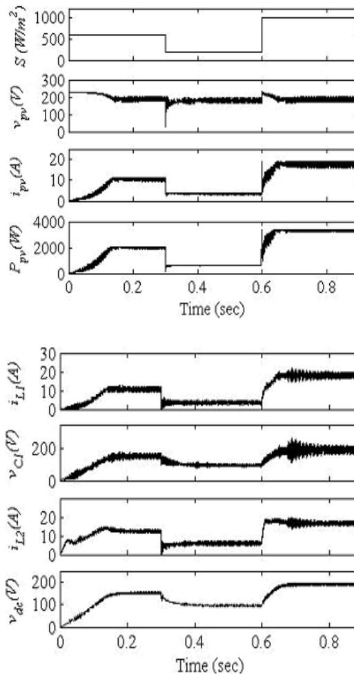
**Fig. 5 Dynamic performances of the proposed SPV array based Zeta converter fed BLDC motor drive for water pump (a) SPV array variables, (b) Zeta converter variables**
