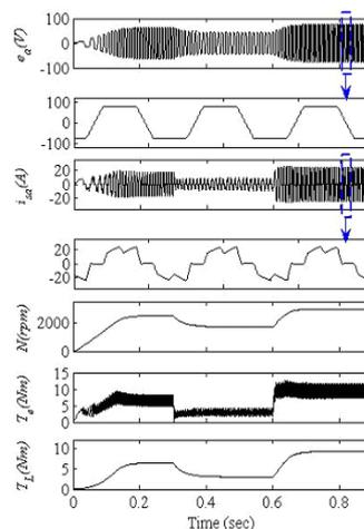
**Fig. 5 Dynamic performances of the proposed SPV array based Zeta converter fed BLDC motor drive for water pump (c) BLDC motor-pump variables.**
