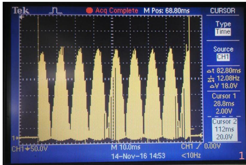
**Image 1: PWM of contactor on 240VAC Application**
