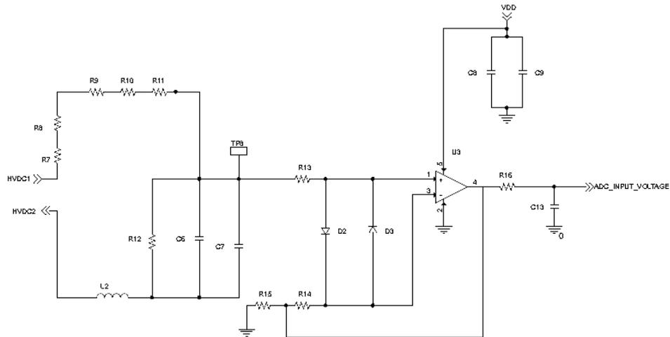
Figure 4: Voltage Detection Circuit.
