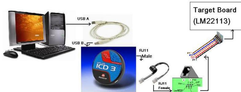
Figure 3: Software process flow & IED installation guide
