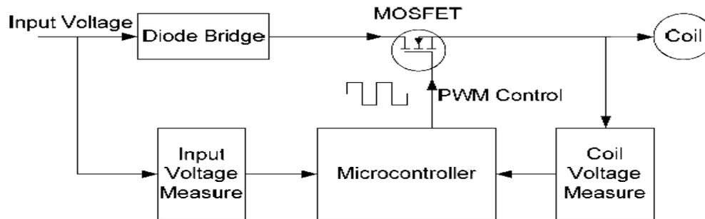
**Figure 1: Principle diagram of system**
