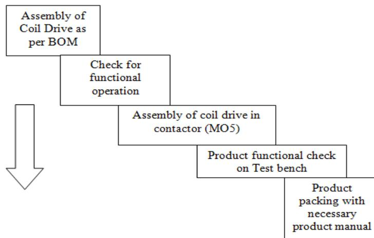
Figure 4: Process flow for MO5 contactor
