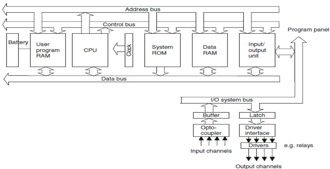
**Fig. 3.2(b): Architecture of PLC.**
