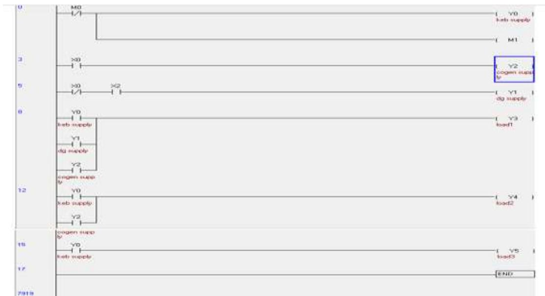
**Fig. 7: Basic ladder program to check the availability of power supply**
