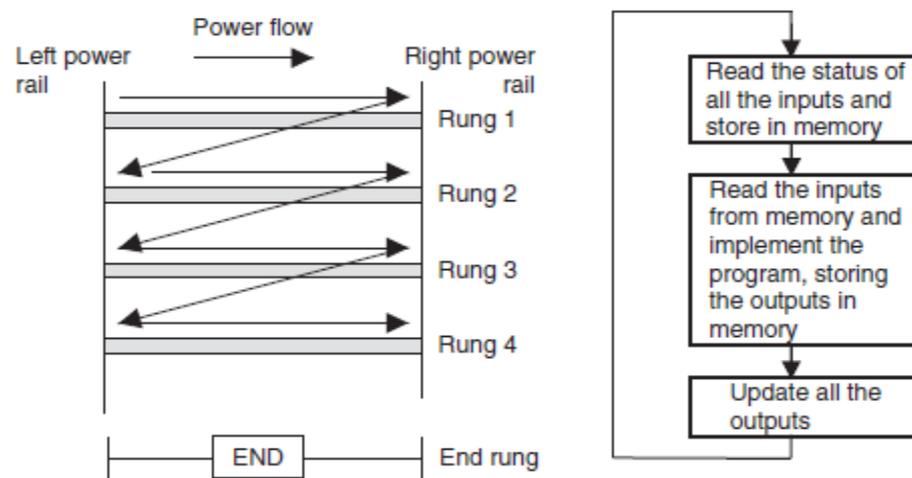
**Fig. 4: Scanning the ladder program**
