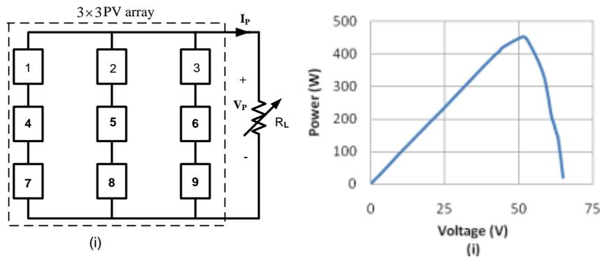
**Fig. 4**  $3 \times 3$  PV Array Configuration Having Nine Panels Connected in Series-Parallel Arrangement. (CASE 1 All Panels are Receiving Insolation of  $1000 \text{ W/m}^2$  at  $25^\circ \text{ C}$ )
