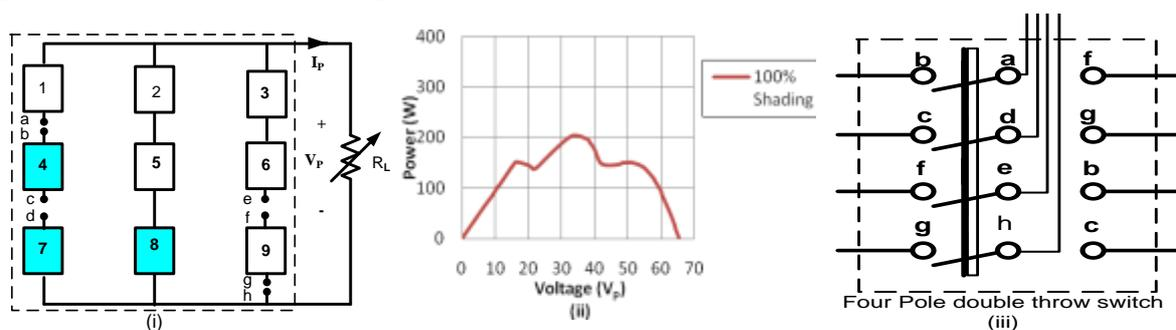
**Fig. 5 (D)  $3 \times 3$  PV Array Showing Configuration Having Nine Panels Connected in Series-Parallel Arrangement with Three Panels (Panel 4, 7 & 8) Shaded (CASE 5). the PV Characteristic is Shown for 100% Shading on Panel 4, 7 & 8.**
