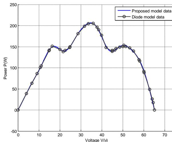
**Fig. 9 The P-V Characteristic Obtained From Single Diode Model and Proposed Model for The Case When Three Panels are Shaded as Shown in Fig. 5(D)**
