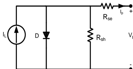
**Fig.2 Single Diode Equivalent Circuit of PV Panel Representing Model Parameters**
