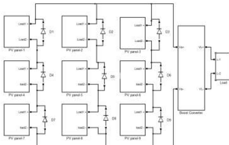
**Fig. 7(A) Simulation Model of 3x3 PV Array Connected in Series Parallel Arrangement and Connected to Load Through Boost Converter**
