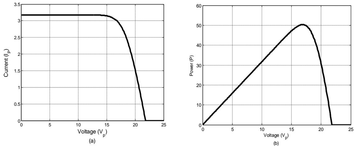
**Fig. 3 I-V and P-V Characteristics of a 50W Solar Panel at Insolation of  $1000\text{W/m}^2$  at  $25^\circ\text{C}$**
