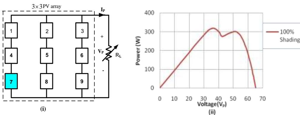
**Fig. 5 (A)** A  $3 \times 3$  PV Array Configuration Having Nine Panels Connected In Series-Parallel Arrangement With One Panel Shaded (CASE 2). PV Characteristic Is Shown For 100% Shading On Panel 7.
