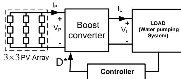
**Fig. 6 Block Diagram Showing PV Array Connected to Load Through Boost Converter**
