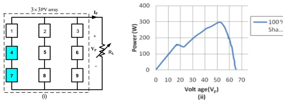
**Fig. 5 (C) A  $3 \times 3$  PV Array Showing Configurations Having Nine Panels Connected In Series-Parallel Arrangement with Two Panels in Series are Shaded (CASE-4). PV Characteristic is Shown for 100% Shading On Panel 4 & 7.**
