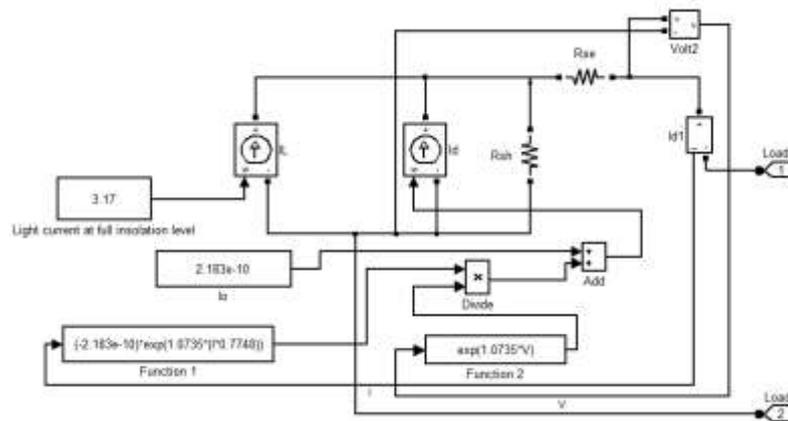
Fig. 7(B) Simulation Model of One PV Panel Fed From Constant Insolation
