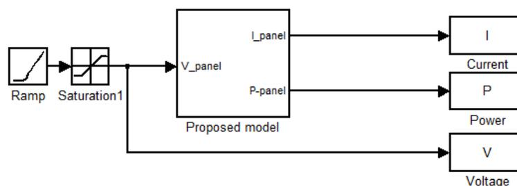
Fig. 8(A) Simulation of Proposed Model of  $3 \times 3$  PV Array Connected in Series Parallel Arrangement When Three Panels are Shaded
