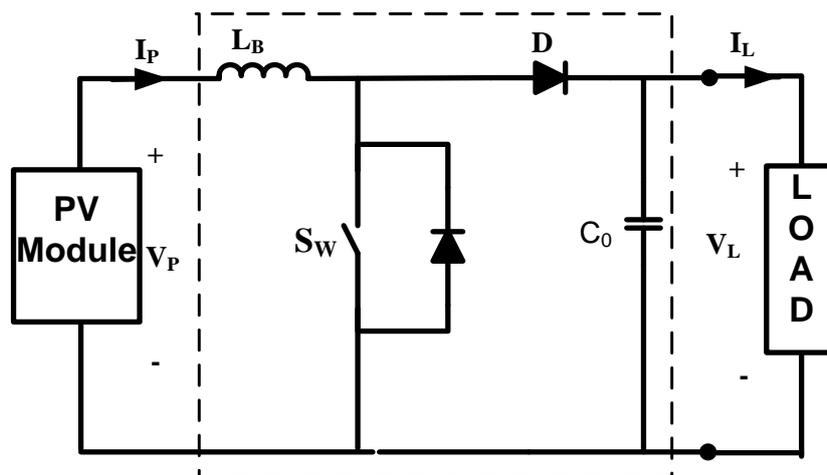
**Fig.1 Circuit Diagram of Boost Converter for Effective Load Matching**
