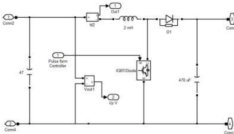
Fig. 7(C) Simulation Model of Boost Converter Employed in The PV Based System
