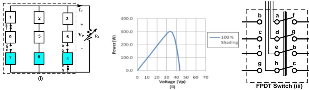
**Fig. 5 (E)  $3 \times 3$  PV Array Showing Configuration Having Nine Panels Connected in Series-Parallel Arrangement with Three Panels (Panel 7, 8 & 4) Shaded (Reconfigured) (CASE 6). The PV Characteristic is Shown for This Case For 100%, Shading on Three Panels.**
