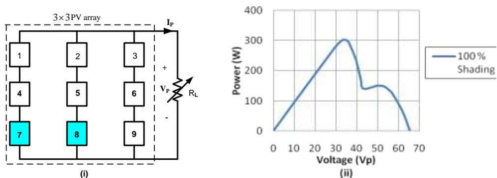
**Fig. 5 (B)** A  $3 \times 3$  PV Array Configuration Having Nine Panels Connected in Series-Parallel Arrangement with Two Panels Shaded (CASE 3). PV Characteristic is Shown for 100%, Shading on Panel 7 & 8.
