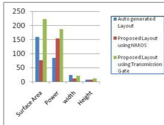
**Fig.8: Layout Comparison for Area, Power and Height**
