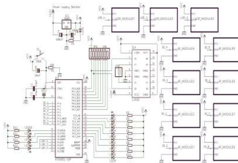
**Fig.7. Circuit Arrangement of Energy Efficient Street Light System**
