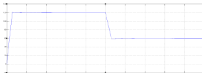
Figure.2The Speed of Separately Excited Direct Current Motor From Initial Speed Zero To Start 120 Rad/Sec After 5 Second The Speed Reach To 120 To 60 Rad/Sec.
