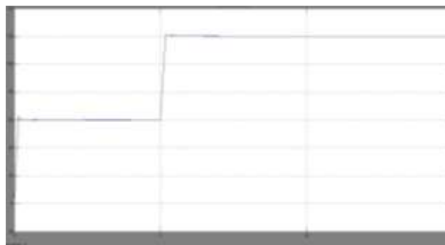
Figure: 4. SEDC Motor Using The (PI) Controller Speeds From Start 60 To 120 Rad/Sec.
