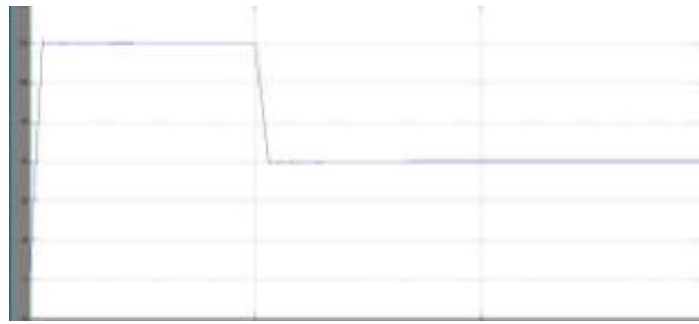
Figure: 7. Shows The Result of SEDC Motor Using The (PI) From 120 To 60 Rad/Sec.
