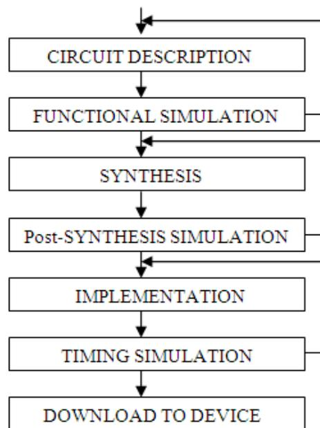
**Fig.2 FPGA Design Flow**
