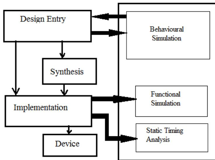
**Fig.1 Block diagram for FPGA simulation Design Entry**
