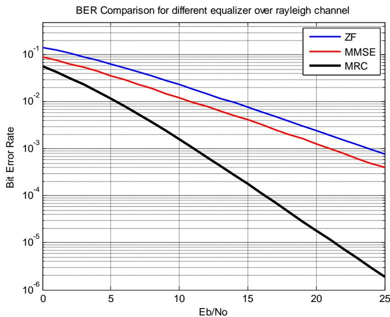
Fig.5.4 Comparison of BER analysis using different equalizer.
