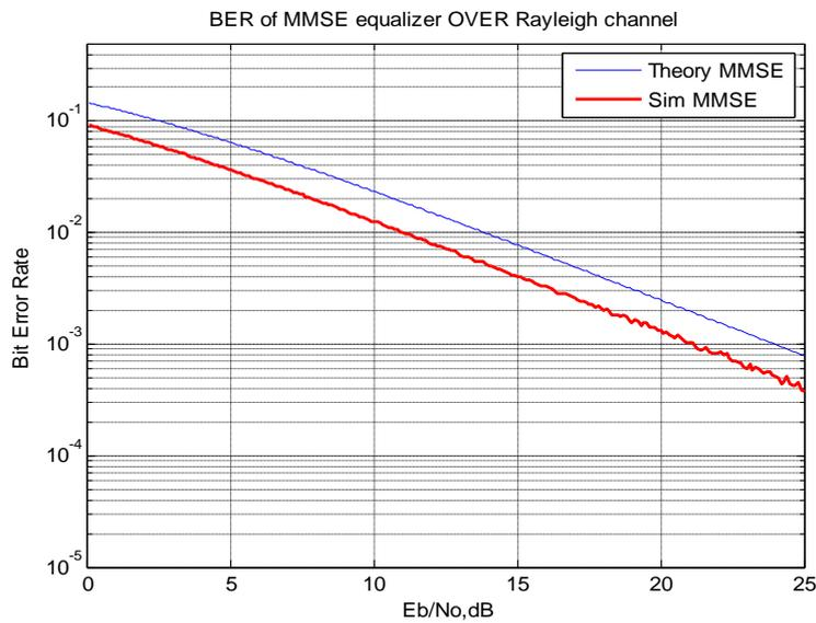
Fig.5.2 BER analysis of MIMO-OFDM system using MMSE equalizer.
