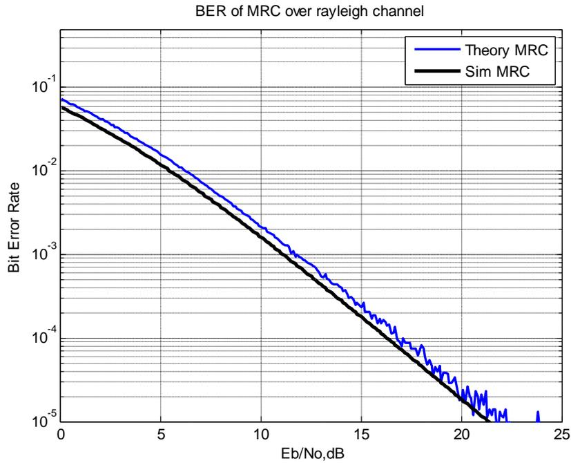
Fig.5.3. BER analysis of MIMO-OFDM system using MRC equalizer.
