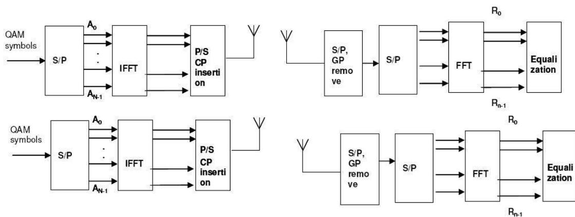
Fig.1. Block Diagram of MIMO- OFDM System
