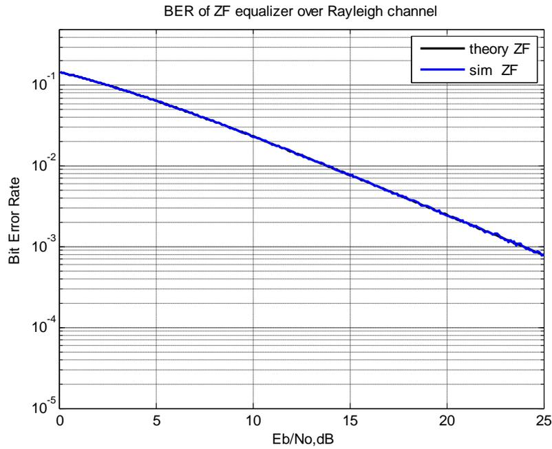
Fig.5..1 BER analysis of MIMO- OFDM system using ZF equalizer.
