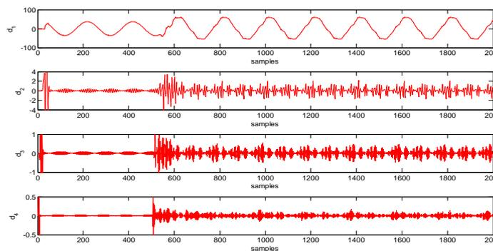
Fig.13 Wavelet Transform of phase-C current signal of Distribution feeder during HIF1 Transients
