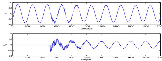
Fig.18 capacitor switching distorted current on phase- A
