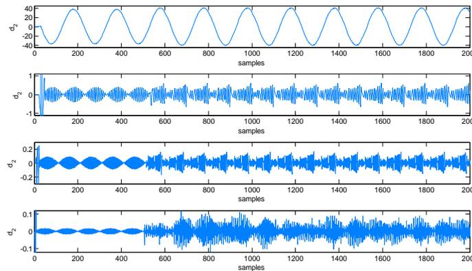
Fig.28 Wavelet Transform of phase-B current signal of Distribution feeder during Non-linear load switching
