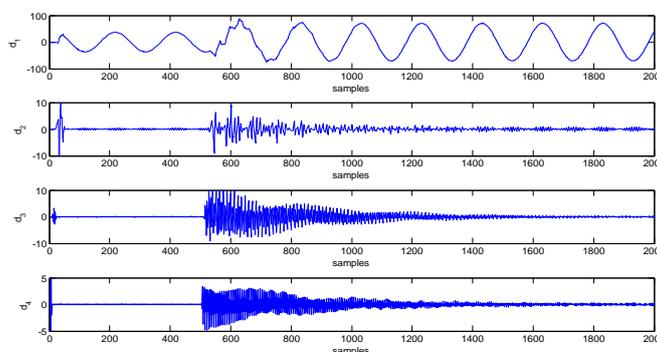
Fig.21 Wavelet Transform of phase-C current signal of Distribution feeder during capacitor switching
