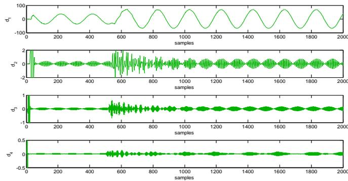
Fig.25 Wavelet Transform of phase-C current signal of Distribution feeder during load switching
