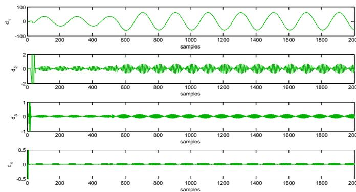
Fig.23 Wavelet Transform of phase-A current signal of Distribution feeder during load switching
