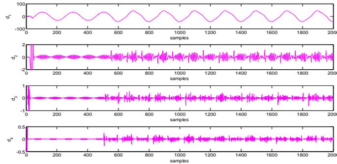
Fig.15 Wavelet Transform of phase-A current signal of Distribution feeder during HIF2 transients
