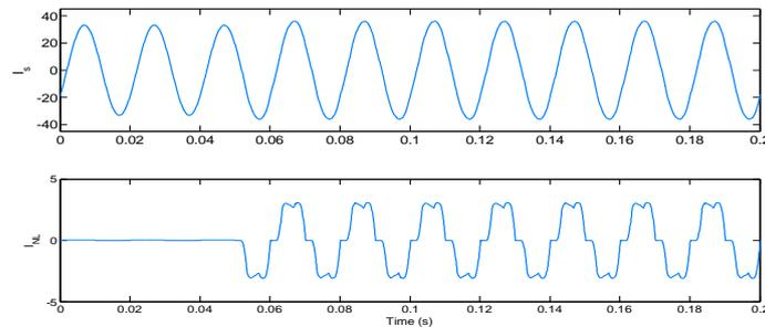
Fig.26 Nonlinear load distorted current on phase A.
