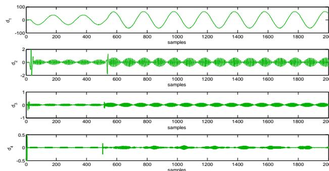
Fig.24 Wavelet Transform of phase-B current signal of Distribution feeder during load switching
