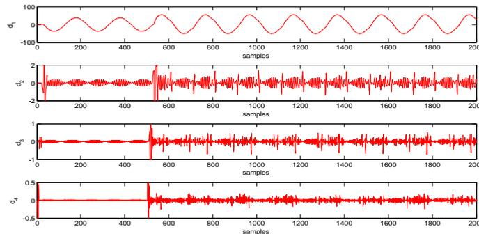
Fig.12 Wavelet Transform of phase-B current signal of Distribution feeder during HIF1 Transients
