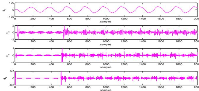
Fig.16 Wavelet Transform of phase-B current signal of Distribution feeder during HIF2 Transients
