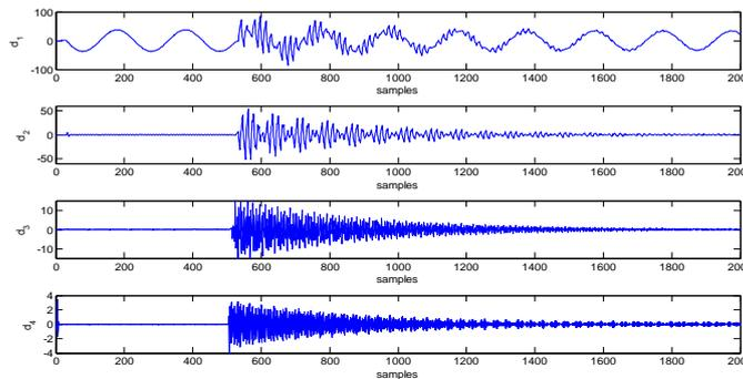
Fig.20 Wavelet Transform of phase-B current signal of Distribution feeder during capacitor switching
