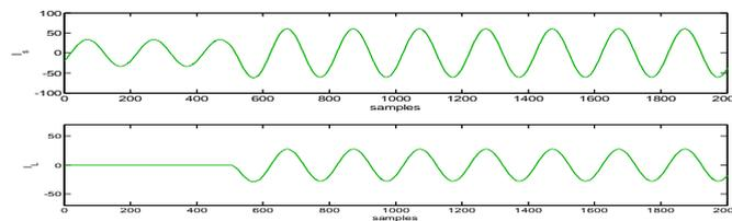
Fig.22 Load switching distorted current on phase A
