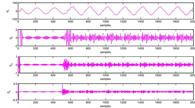
Fig.17 Wavelet Transform of phase-C current signal of Distribution feeder during HIF2 Transients
