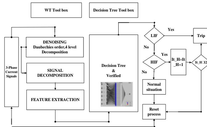
Fig. 1.Schematic diagram of the methodology
