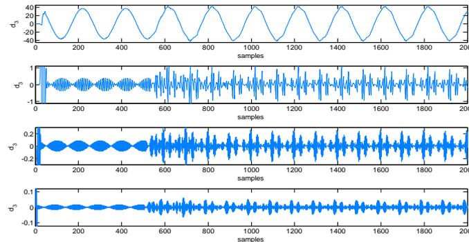
Fig.29 Wavelet Transform of phase-C current signal of Distribution feeder during Non-linear load switching
