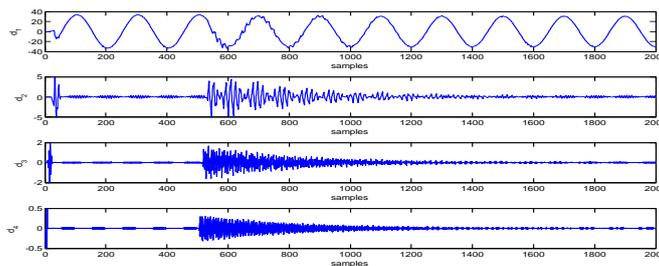
Fig.19 Wavelet Transform of phase-A current signal of Distribution feeder during capacitor switching
