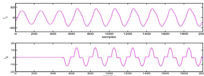
Fig.14 High Impedance Fault 2 distorted current on phase A.
