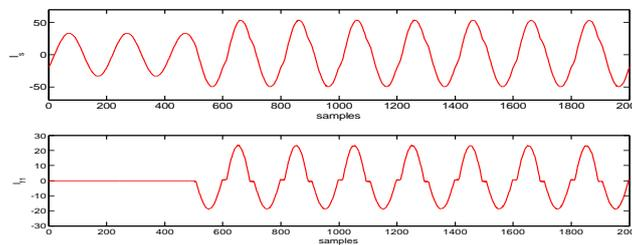
Fig. 10 High Impedance Fault 1 distorted current on phase- A
