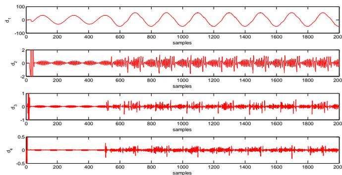
Fig. 11 Wavelet Transform of phase-A current signal of Distribution feeder during HIF1 Transients
