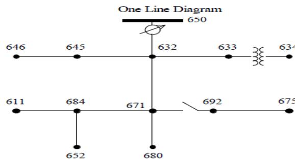
Fig.8 13 Node IEEE Test Feeders
