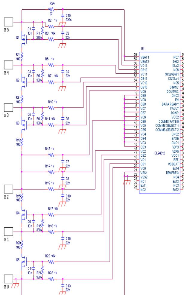
Fig: connection of battery pack and monitoring Ic
