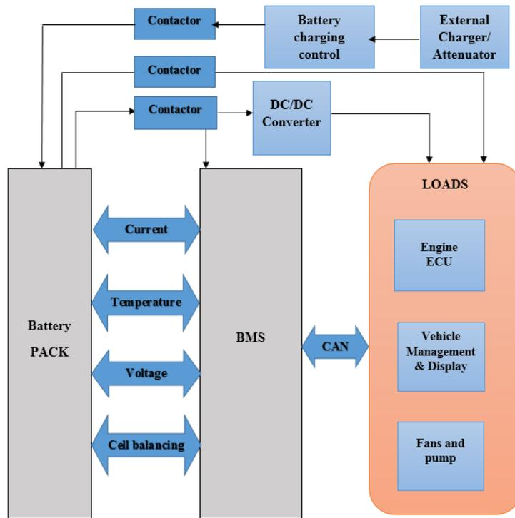
Fig: Basic block diagram of BMS
