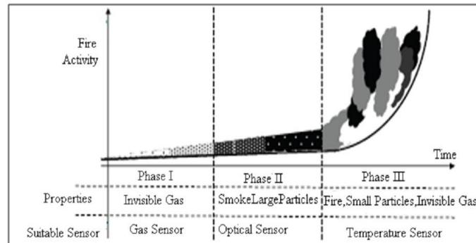
Fig.5 Fire Characteristics diagram
