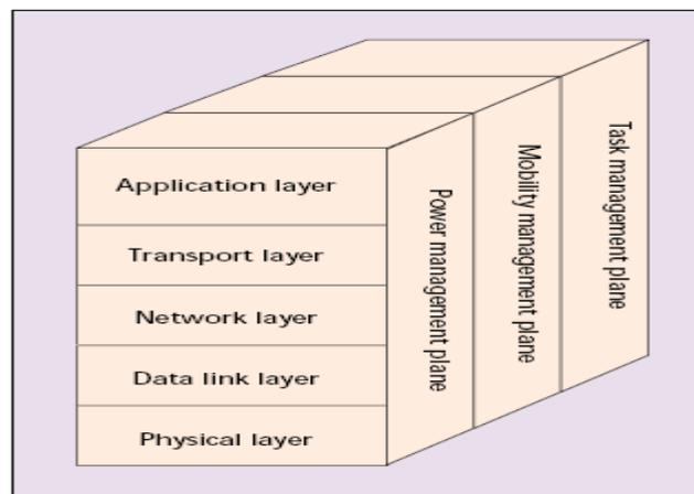
Fig 2. Wireless Sensor Network Protocol Stack
