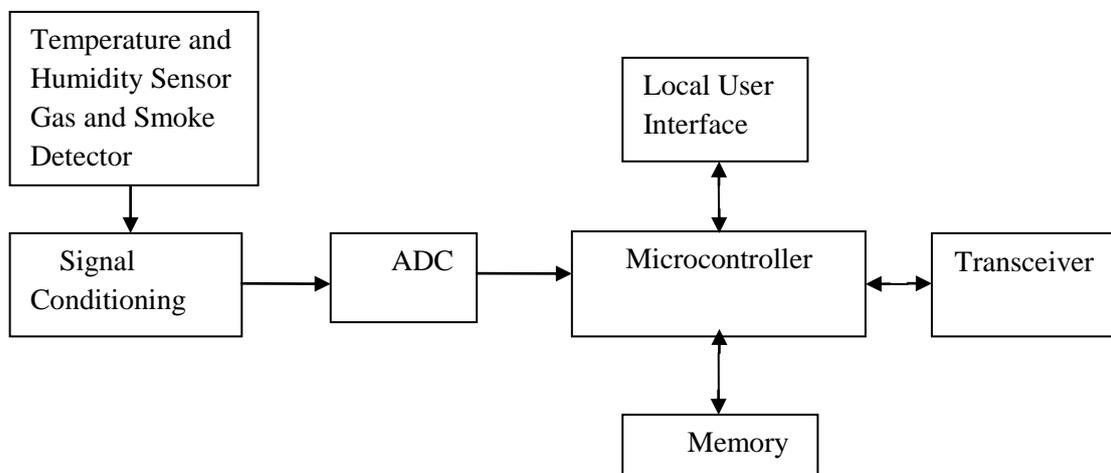
Fig.3 Components of a Sensor node
