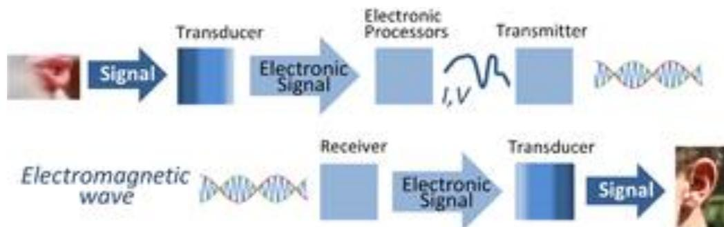
Transducing information such as sound into an electromagnetic pulse signal, which is then sent as an electromagnetic radio wave from a transmitter. A receiver intercepts the radio wave and extracts the information-bearing electronic signal, which is converted back using another transducer such as a speaker.
