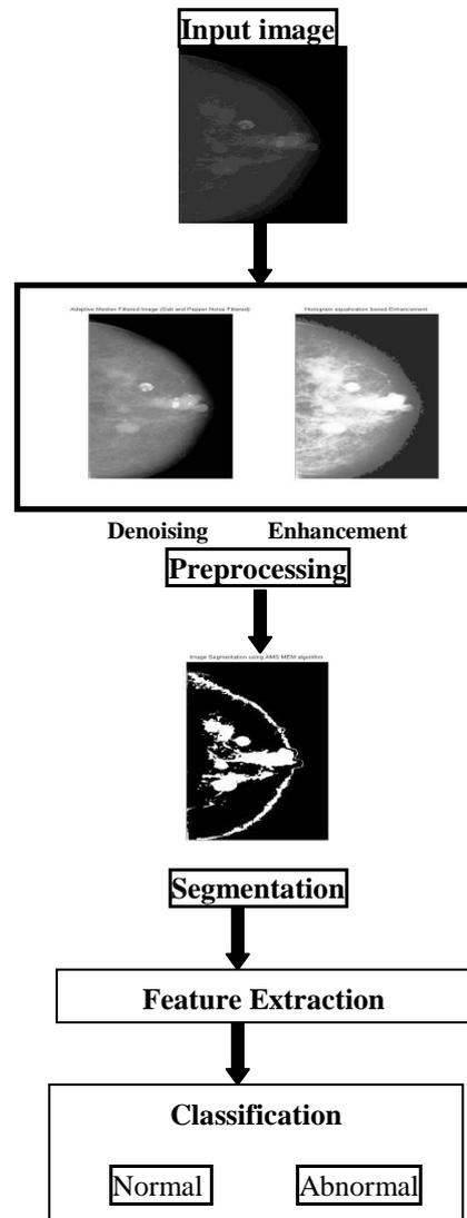
**Figure 2. Block Diagram**
