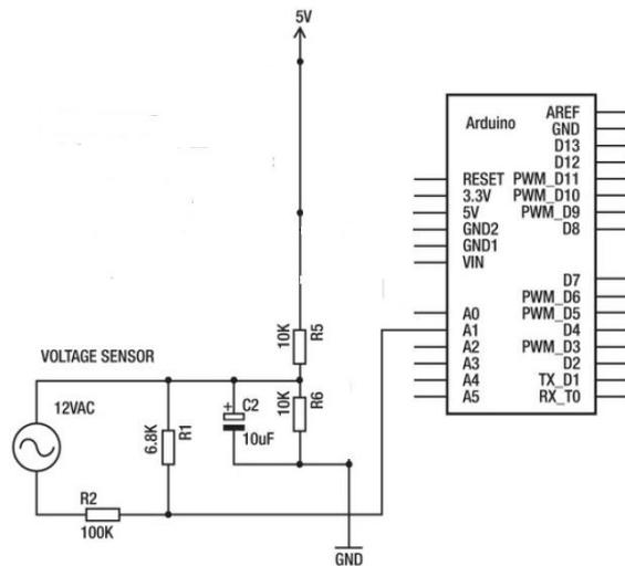
**Figure 2: Voltage Sensor**
