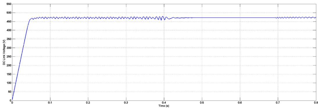
**Fig. 7 input of the inverter which is the output of PV cell**
