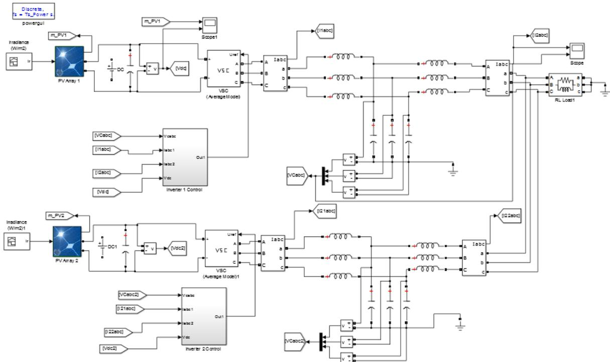
**Fig.4 Model of grid connected microgrid using droop method in MATLAB**
