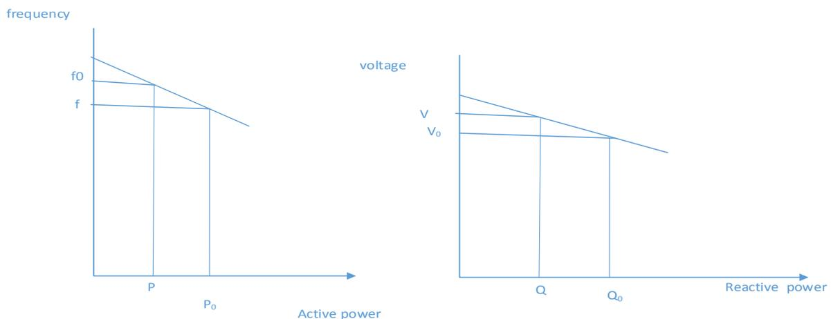
**Fig. 2 droop voltage and droop frequency characteristic**
