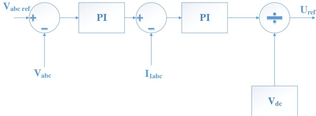
**Fig. 3 Block diagram of voltage and current control design**
