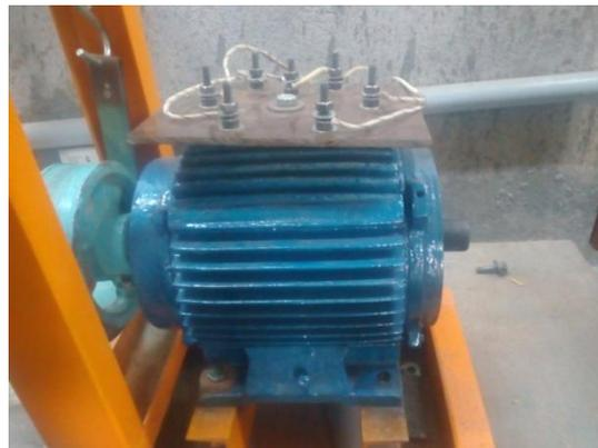
**Fig.6 Phase Induction Motor**
