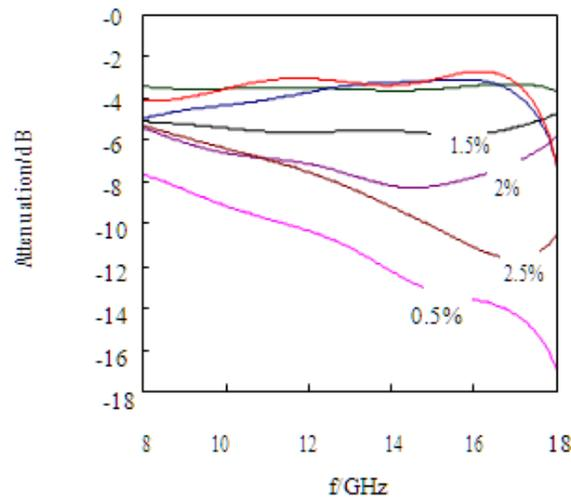
**Figure. 1: The absorbing performance of CBCC with different concentration of CB in the frequency range of 8–18 GHz.**
