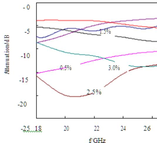
**Figure. 2: The absorbing performance of CBCC with different concentration of CB in the frequency range of 18-26.5 GHz.**
