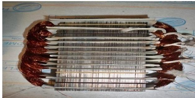
**Fig.1.5: Primary stack formation with windings**
