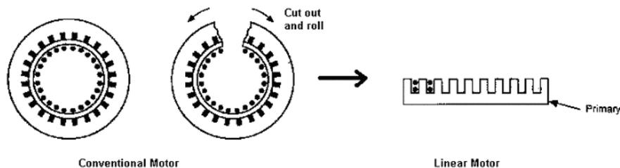
Fig. 1.1: Visualization of LIM from rotary induction motor
