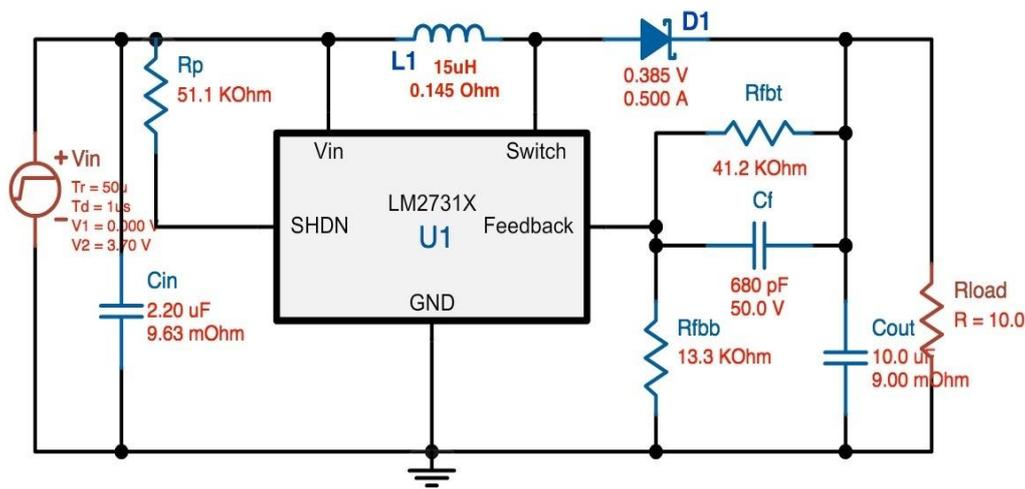
Fig 4.1 LM2731 boost converter
