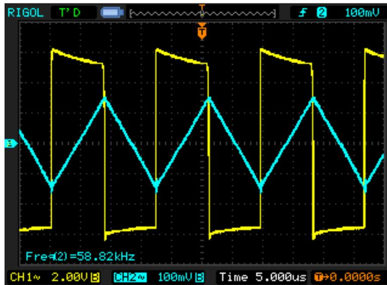
Fig 7.4 Ripple at 5V,1A
