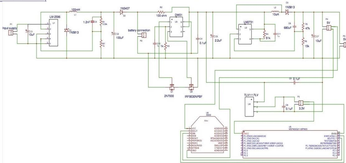
**Fig 2.2 Schematic diagram**
