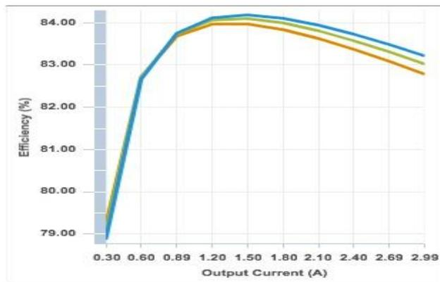
Fig 3.3 Efficiency variation with respect to load current
