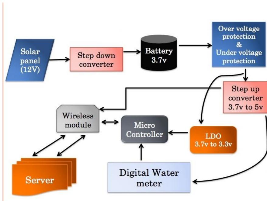
**Fig 2.1 Block diagram**
