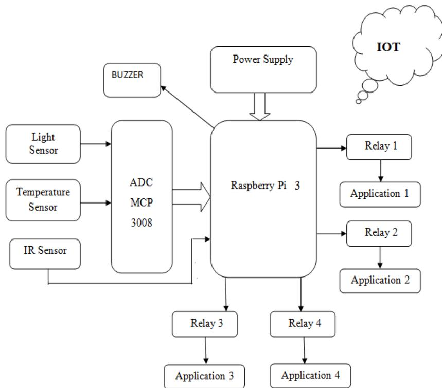
**Fig.3 Block Diagram of industrial Automation System by Using Raspberry Pi**
