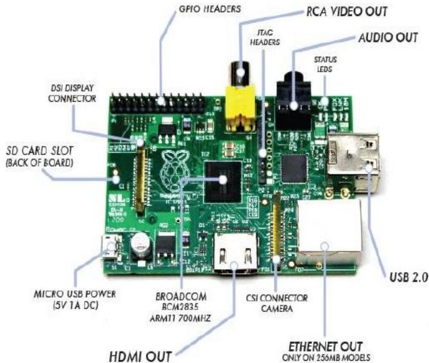
**Fig.2 Raspberry Pi Microcontroller Board**
