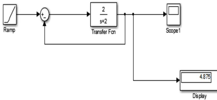
**Figure13:Simulink model for Ramp first order with feed back**
