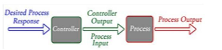
**Figure 1:Block diagram of Open loop Control System**
