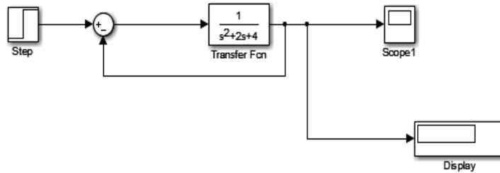
Figure 9: Simulink model for Second Order with feed back
