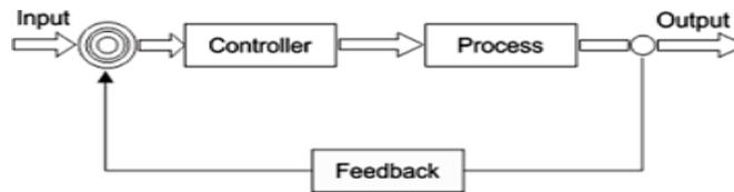
**Figure 2 Block diagram of Closed loop Control System**
