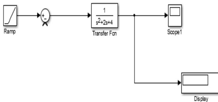
**Figure15:Simulink model for Ramp Second order without feed back**
