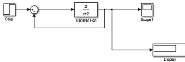
**Figure 5: Simulink model for first order with feedback**
