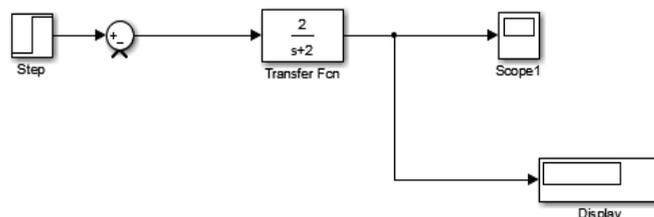
**Figure 3:Simulink model for first order without feed back**
