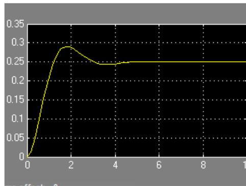
Figure 10. Unit Step second Order System without Feedback
