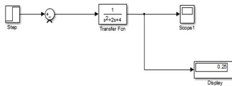
**Figure 7: Simulink model for second order without feedback**
