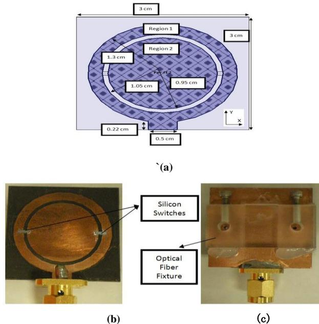
Fig. 3 (a) The stripline fed structure of antenna (b) The top view of antenna prototype (c) The antenna prototype in bottom view [6]
