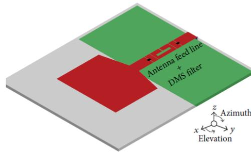
**Fig.7 The Reconfigurable filtenna Concept**
