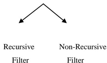
The response of non-Recursive or FIR filters depend only upon Present and previous input of signal. The response of Recursive or IIR filters depends on present inputs, past inputs and previous outputs also.
