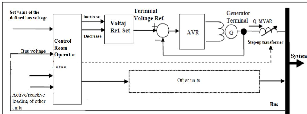
**Figure no.2 Control via an Operator**
