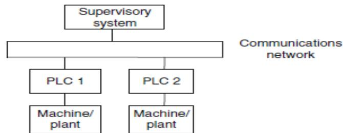
**Fig. 3.2(a): Basic communication model.**
