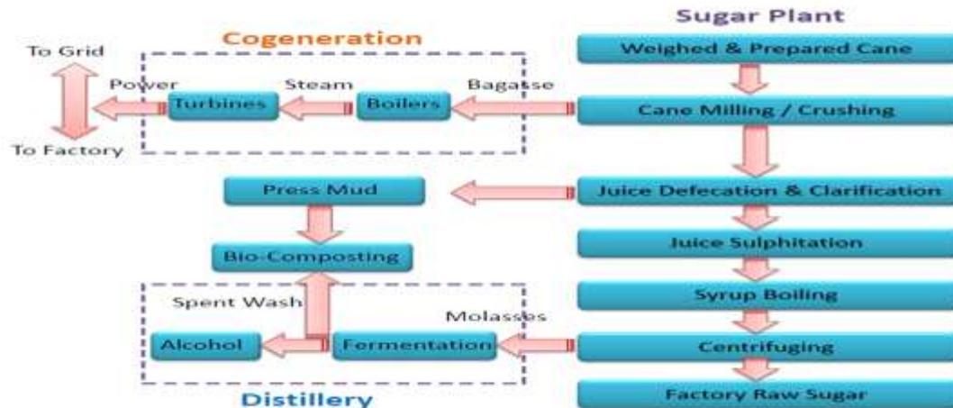
The process flow in sugar industry is shown in Fig. 6.
