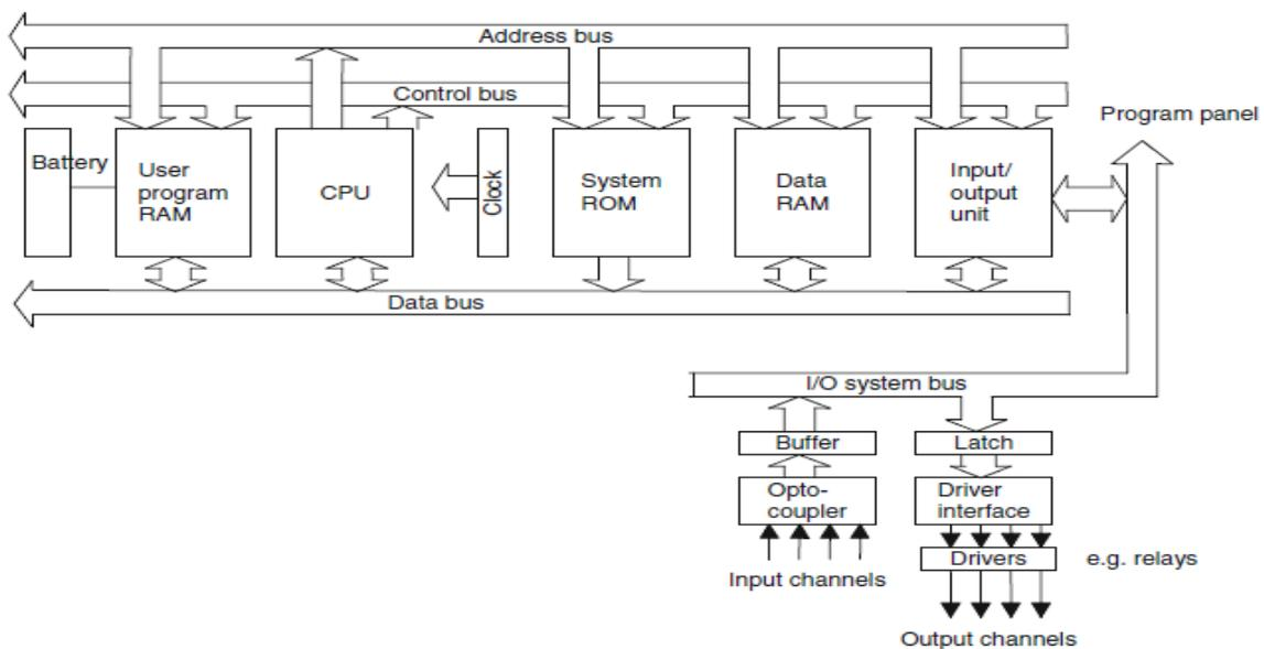
**Fig. 3.2(b): Architecture of PLC.**
