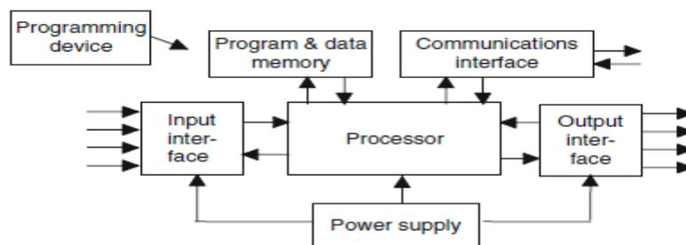
**Fig. 3: The PLC System**
