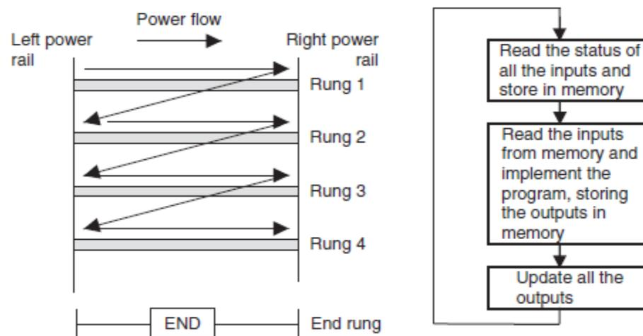
**Fig. 4: Scanning the ladder program**
