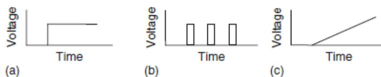
**Fig. 3.1: Signals: (a) discrete, (b) digital, and (c) analog.**
