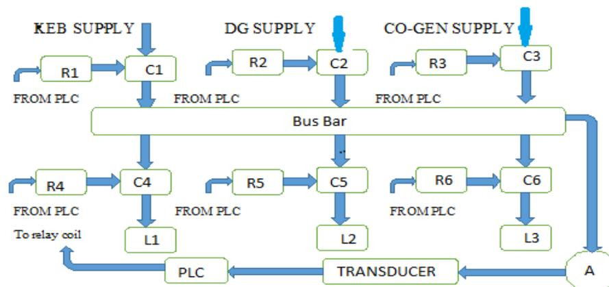
**Fig. 1: Block Diagram of Load Management in Sugar Industry Using PLC**
