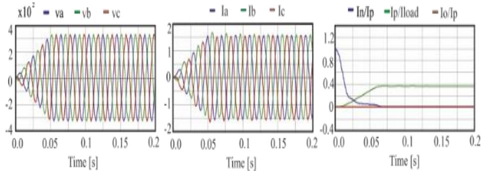
Figure 2: Normal conditions: three phase voltages ( $V$ ), three phase current in ( $A$ ) the ration of sequence components of currents
