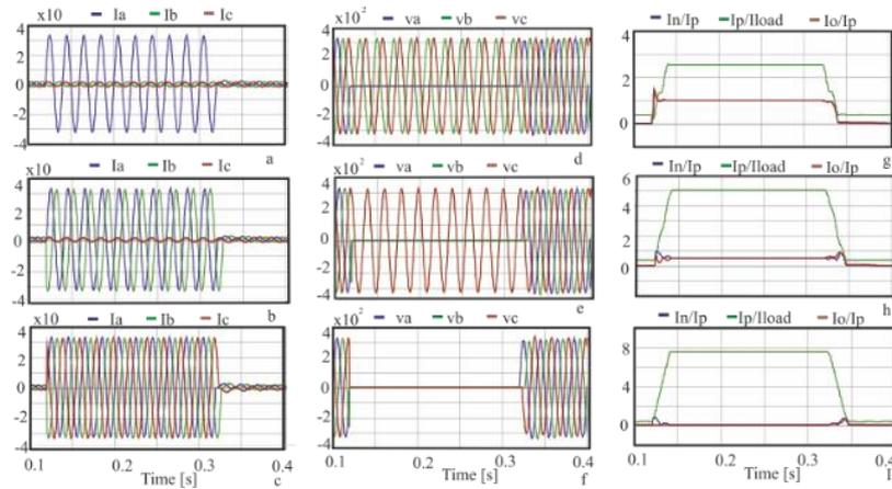
Figure 4: Fault simulation at **0km** location on transmission line with **g, h** and **i** represent the ratio of sequence components currents for three line to ground, Double line to ground and single line to ground fault respectively.
