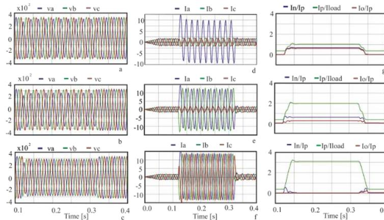
Figure 5: Fault simulation at **50km** location on transmission line **d, e** and **f** representing the instantaneous currents during single line to ground, Double line to ground and three line to ground fault respectively.
