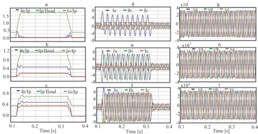
Figure 3: Fault simulation at **100km** location on transmission line with **a**, **b** and **c** represent the ratio of sequence components currents for three line to ground, Double line to ground and single line to ground fault respectively. **d**, **e**, **f** and **g**, **h**, **i** represent the instantaneous currents and voltages during single, double and three lines to ground faults (fault start at **120ms** and duration **0.2s**) respectively.
