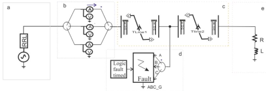
Figure 1: The studied model in PSCAD (fault location at  $50km$ ) : (a) generator of  $400kV$  (b) multimeter (c)  $100km$  transmission line (d) fault module and (e) load
