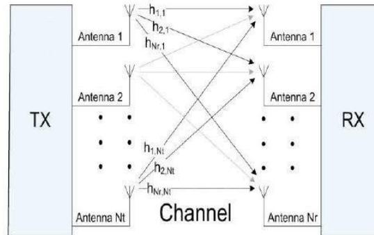
Summation= $\text{diag}(\sigma_{1,2,r,0,\dots,0})$ . Thus, the MIMO channel can be decomposed into  $r$  independent SISO channel has a gain  $\sigma_i$  and a noise factor  $v_i$ , and assumes the representation. This implies all the efficient signaling and decoding strategies well investigated in the SISO context could be transferred mutatis-mutandis to the MIMO framework with a minimal effort.
