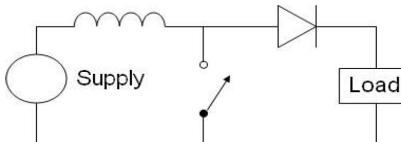
**Fig 1:** basic structure of boost converter
