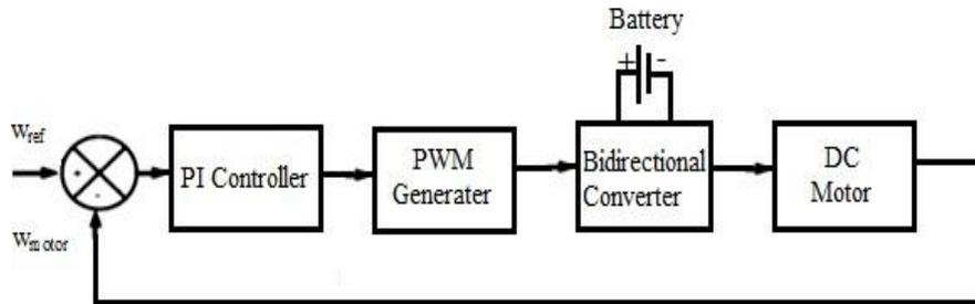
**Fig. 4:** Closed loop operation of the drive.
