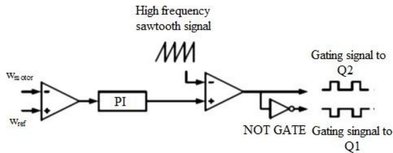
**Fig. 3:** Control strategy of the bidirectional dc-dc converter.
