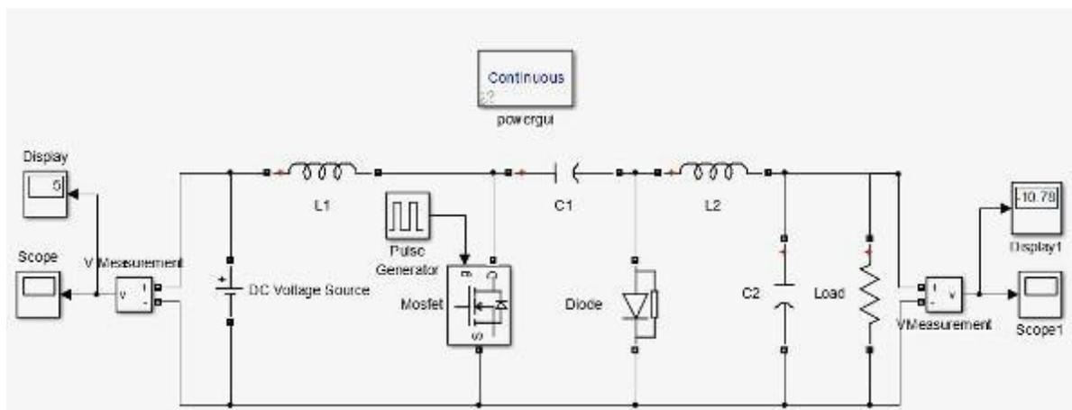
**Fig 8: Cuk converter Simulink model**
