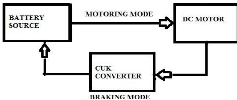
**Fig 12:** Block diagram of Two wheeler system
