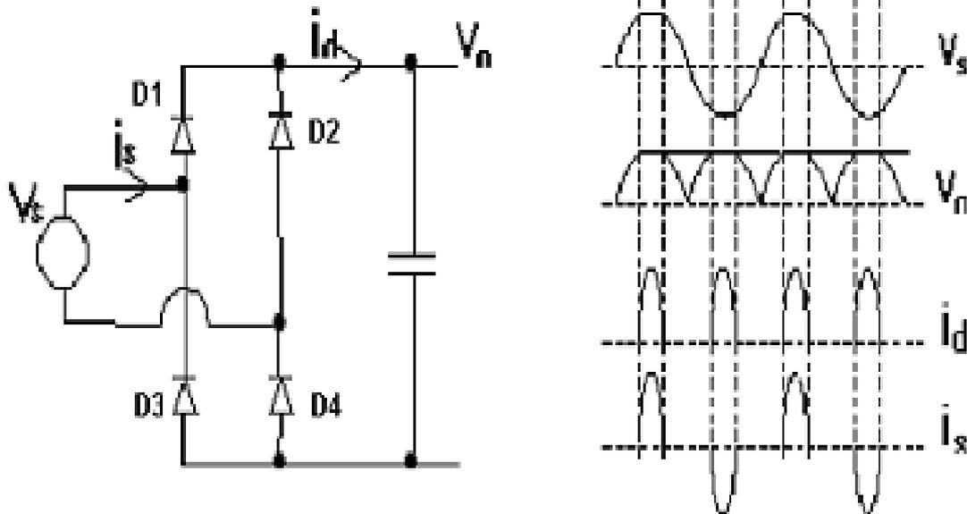
Fig.9.DIODE BRIDGE RECTIFIER
