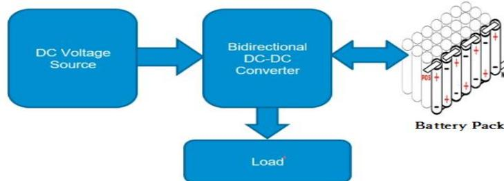
Fig.5 Converter and Battery Arrangement
