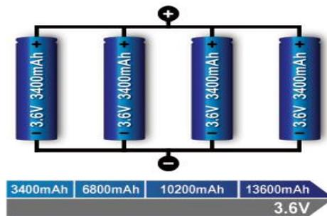
Fig.2 Parallel Connection
