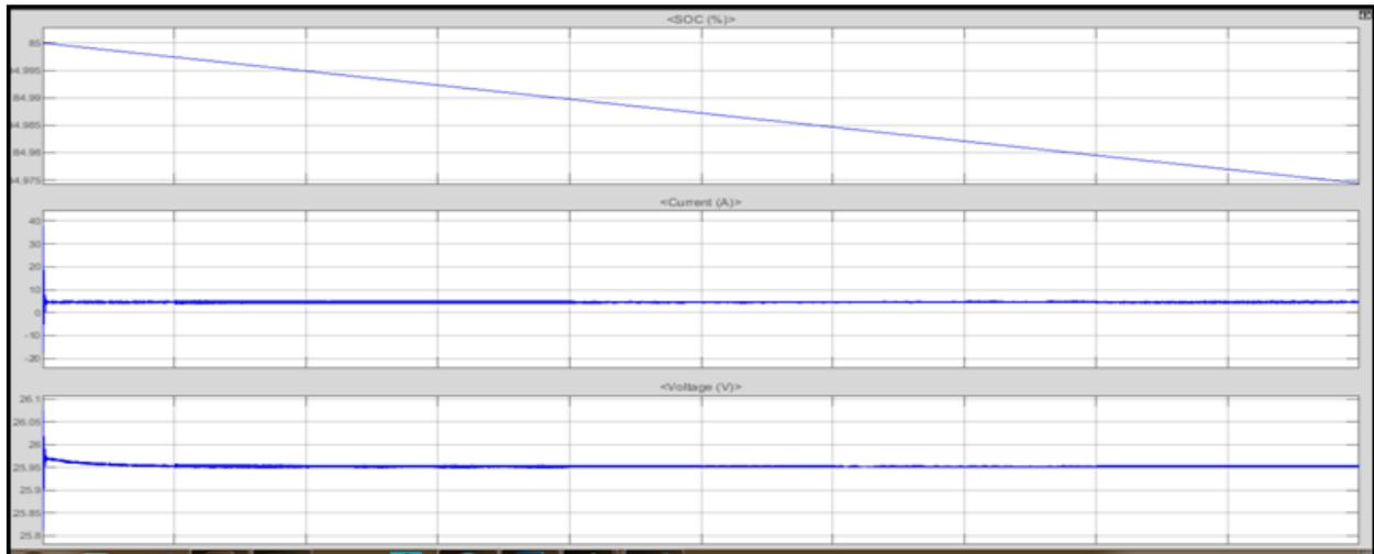
Fig. 12. Simulink output - discharging state of the battery at constant voltage mode
