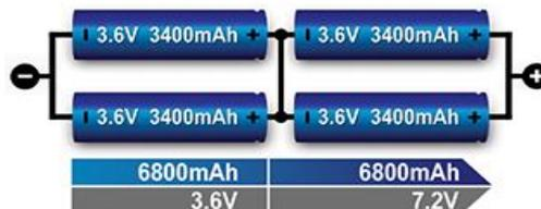
Fig. 3 Series and Parallel Connection
