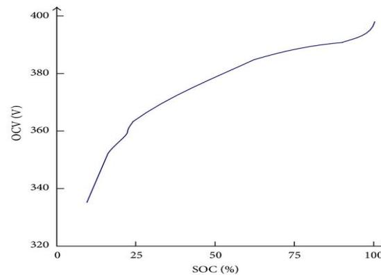
Fig.4.Non linear relationship between OCV and SOC for a lithium ion battery
