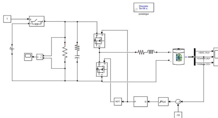
Fig 6. Simulink block for constant current mode
