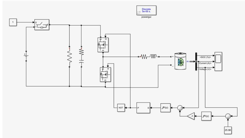
Fig.7. Simulink block for constant voltage of operation
