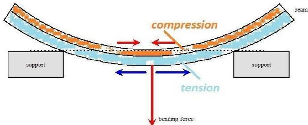
**Fig:1 Stress Bending**
