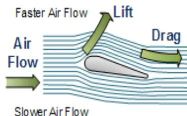
The pressure at the lower surface is greater and thus acts to “lift” the blade upwards, so we want to make this force as big as possible. When the blades are attached to a central rotational axis, like a wind turbine rotor, this lift is translated into a rotational motion.
