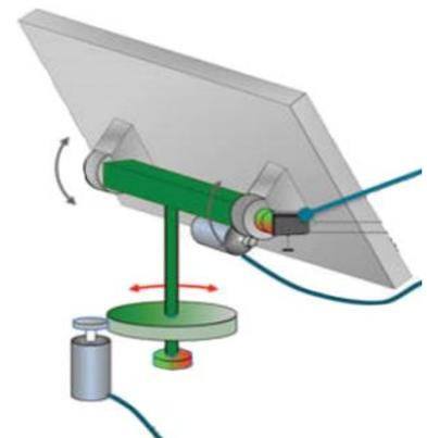
**Fig. Proposed solar tracking set up**
