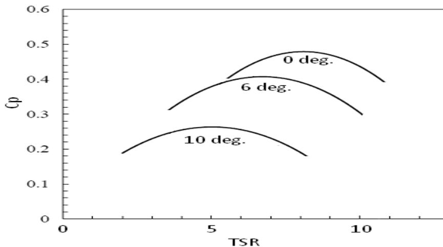
Fig.-Power coefficient Vs Tip Speed Ratio with Angle Of Attack.
