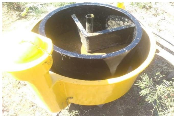
Fig6; Digester Inner side
