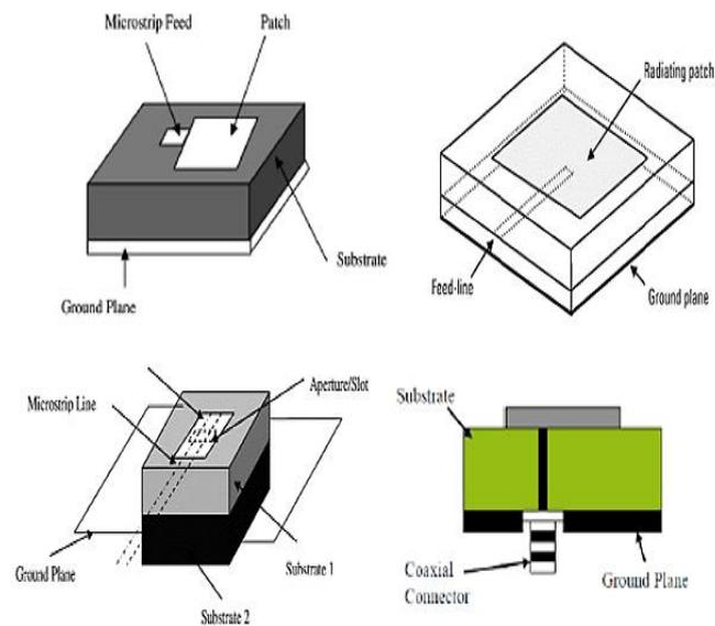
Fig 3: Microstrip Feeds: (a) Line feed (upper left); (b)proximity-coupling (upper right); (c) Aperture-coupling feed (lower left); and (d) Co-axial Feed (lower rt) [21]
