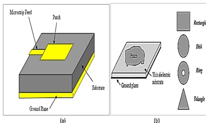
Fig1: (a) Basic Structure of Microstrip Patch Antenna [16]; (b) fundamental configuration of the MPA [17].
