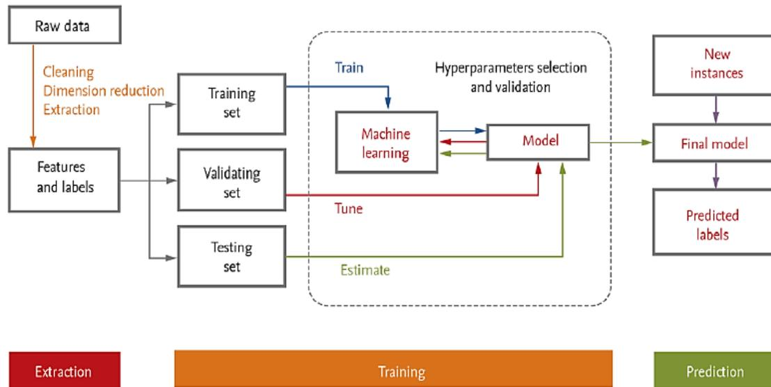
Fig 6: Workflow to develop a supervised machine-learning-based predictive model for antenna design process
