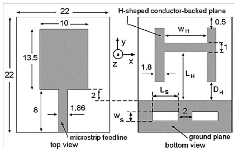
Fig 4(a): Geometry of Planar Monopole Antenna [23]
