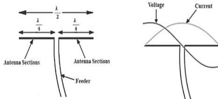
Fig3c: Basic half wave dipole antenna (left) and  $I$  and  $V$  distribution in a half-wave dipole antenna [16]
