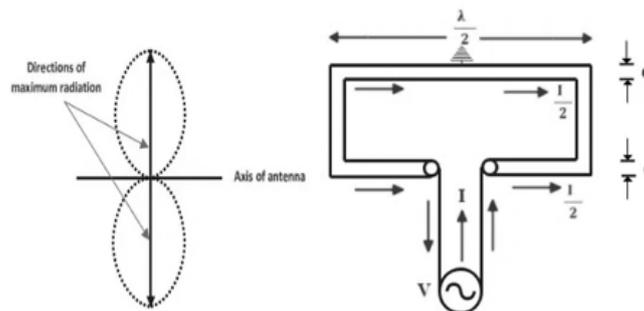
Fig1: Basic dipole antenna and its movement [16]
