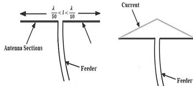
Fig 3d: Short Dipole Antenna (left) and Current Distribution in a Short Dipole Antenna [16]
