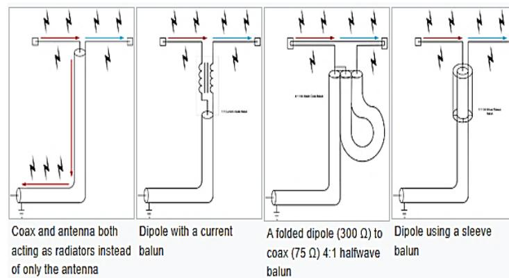
Fig6: Feeding a dipole antenna with coax cable[18]
