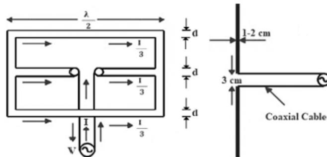
Fig 3a: Folded Tripole Antenna (left) and FM Dipole Antenna (right) [16]
