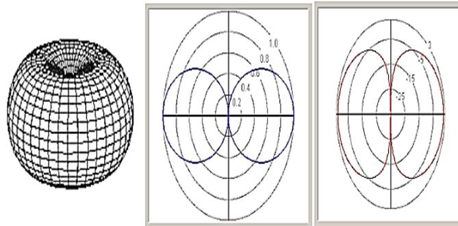
Fig5: 3D radiation pattern of a vertical half-wave dipole antenna (left); Radiation pattern of vertical half-wave dipole; vertical section (center) In linear scale (right) In decibels isotropic (dBi) [20]
