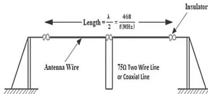
Fig 2: 1 MHz Dipole Antenna Design [16]
